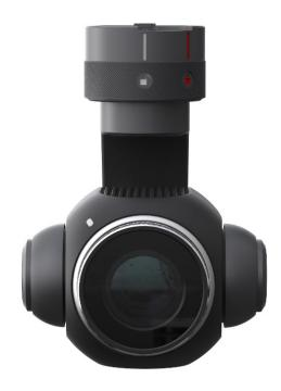
The E90X is a wide-angle high resolution payload/camera for the H520E, Featuring a 1" CMOS sensor, capable of capturing 20MP stills and 100MBPs video (4K at 60FPS). The E90X features a a 90° FOV and a rolling shutter, ideal for mapping applications.
